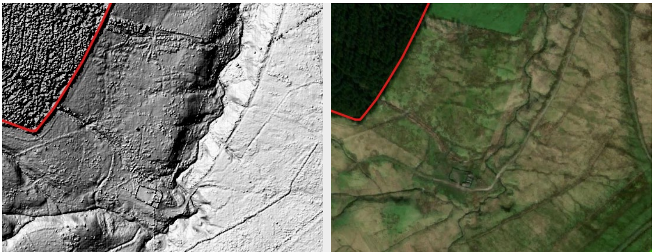
Figure Insert 3.2: LiDAR imagery (left) and aerial imagery (right) illustrating watercourse features (image of Back Burn)
