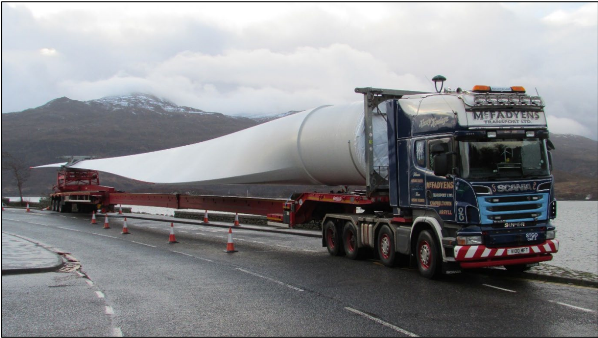
Figure 2 Super Wing Carrier with Loaded Turbine Blade
