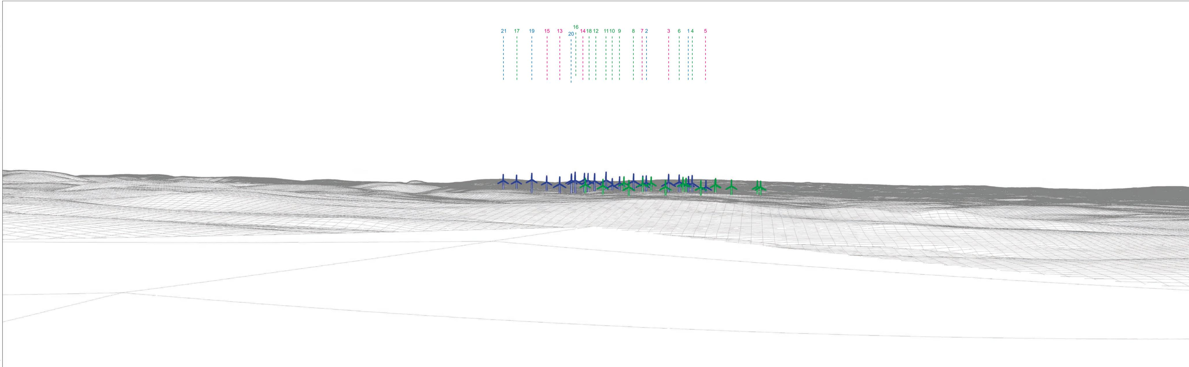
Wireline drawing - left to right: Bloch (11.7km), Solwaybank (9.7km), - Hub / Blade tip height: 105m / 180m (21,19,20,2,1), 125m / 200m (15,13,14,7,3,5), 155m / 230m (17,16,18,12,11,10,9,8,6,4)
